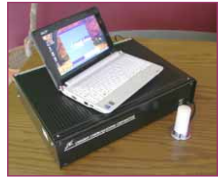
Antenna delivered with 50 ft. cable. Install antenna as high as possible for maximum paging range (1 to 10 miles depending on terrain and antenna height).
